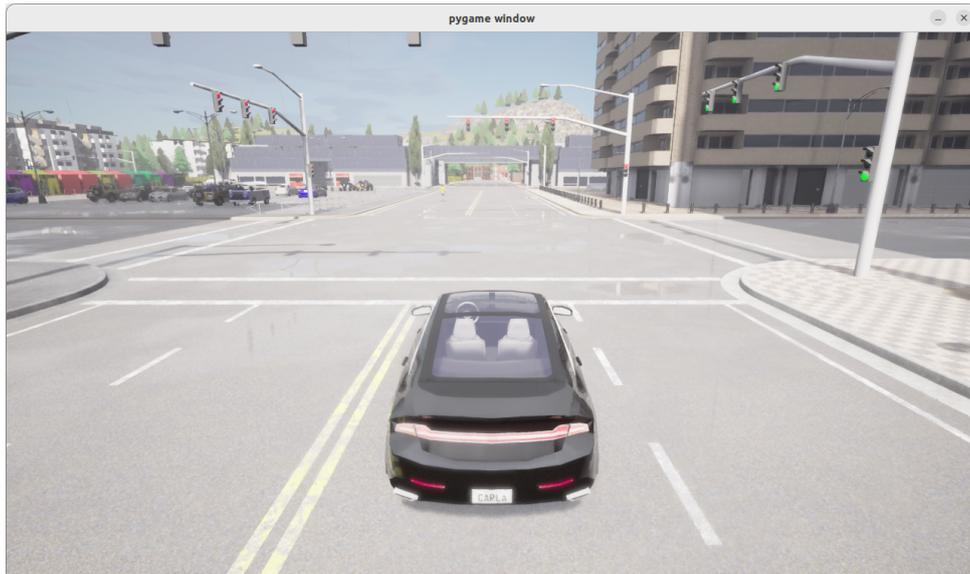
Figure 6: Failed generation example: the Ego car stops but fails to restart even though the pedestrian is far away (and still incorrectly positioned inside the road rather than on the sidewalk).
